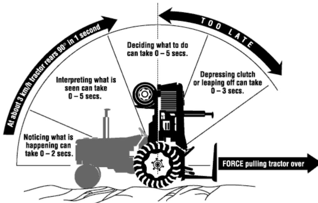
Factors that cause a tractor to tip over backward depend upon the load and the height of the hitch from the ground.
